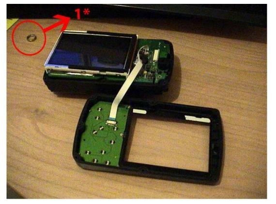
Carefully lift the aluminum paper behind the LCD screen (don't worry it has only soft glue)
