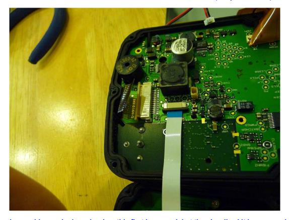
"I may have said some bad words when this first happened, but then I realized it is supposed to do that. I pulled the clamp (for lack of a better term) out of the receptacle, slid the ribbon in and pushed the clamp in to lock it in place (see photo below)."
