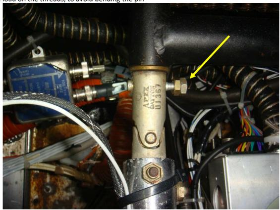
Install the chain breaker – note the clearance from the control sprocket. This is why the collet is needed.
