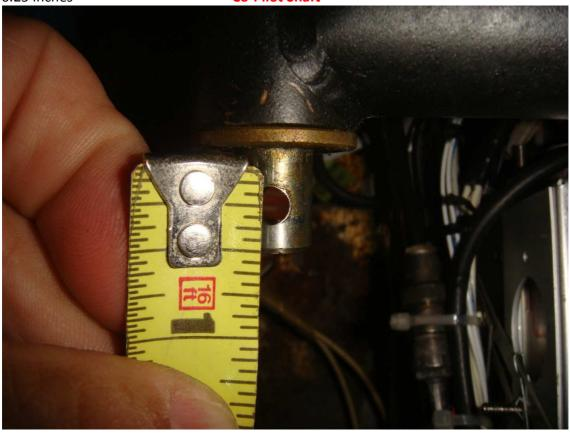
New tapered pin, washer and nut installed. (A new tapered pin and washer are not required per AD/SB)
