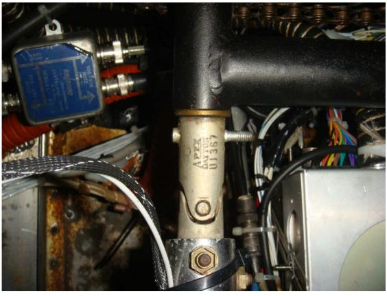
I installed 2 nuts, flush with the tapered pin to provide a pressing surface for the chain breaker and to
