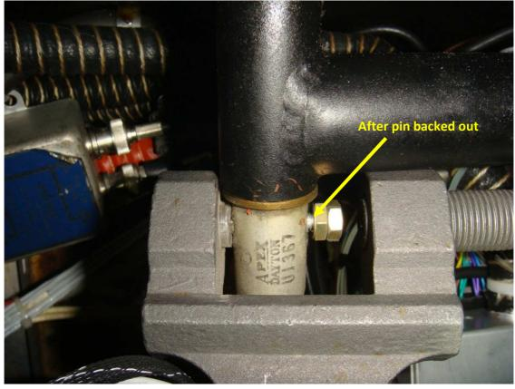
Tapered pin removed – ready for inspection
