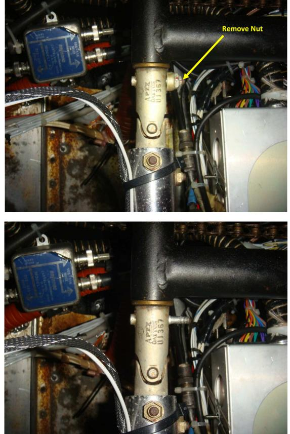
I installed 2 nuts, flush with the tapered pin to provide a pressing surface for the chain breaker and to spread the load on the threads, to avoid bending the pin
