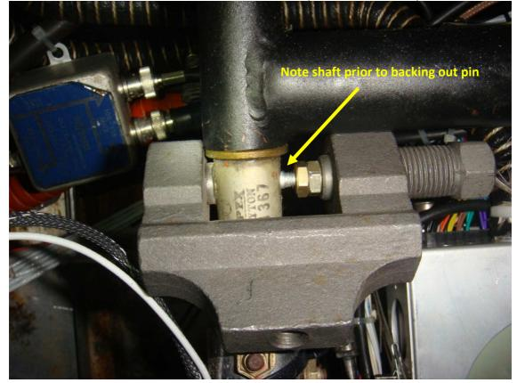
Using a 9/16" wrench or socket, slowly compress the pin, until it releases. In my experience, it required only moderate force. In this picture, the pin has been backed out – note the thread.
