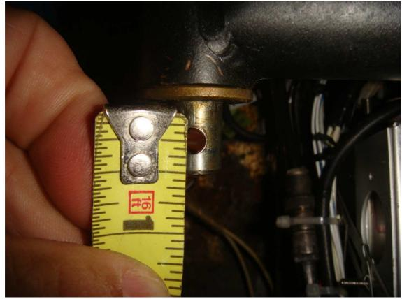
New tapered pin, washer and nut installed. (A new tapered pin and washer are not required per AD/SB)
