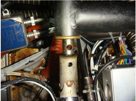
Center of tapered pin hole to end of shaft must be a minimum of 0.19 inches – mine both measured 0.25 inches
